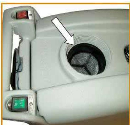
**GB:** Pull the plug of the mains lead out of the socket. Pour the recommended detergent/cleaning liquid in the clean water container.
