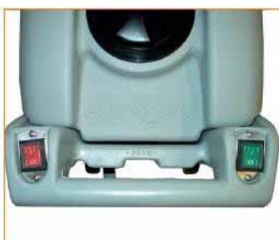
**GB:** It's possible to use the machine to suck liquids only, it's enough to put the green switch in the position «O» (pump not working) and the red switch in position «|».
