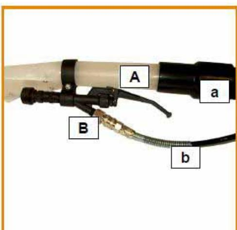
**GB:** Connect tube marked "a" to position marked "A", and connect tube marked "b" to position marked "B".
