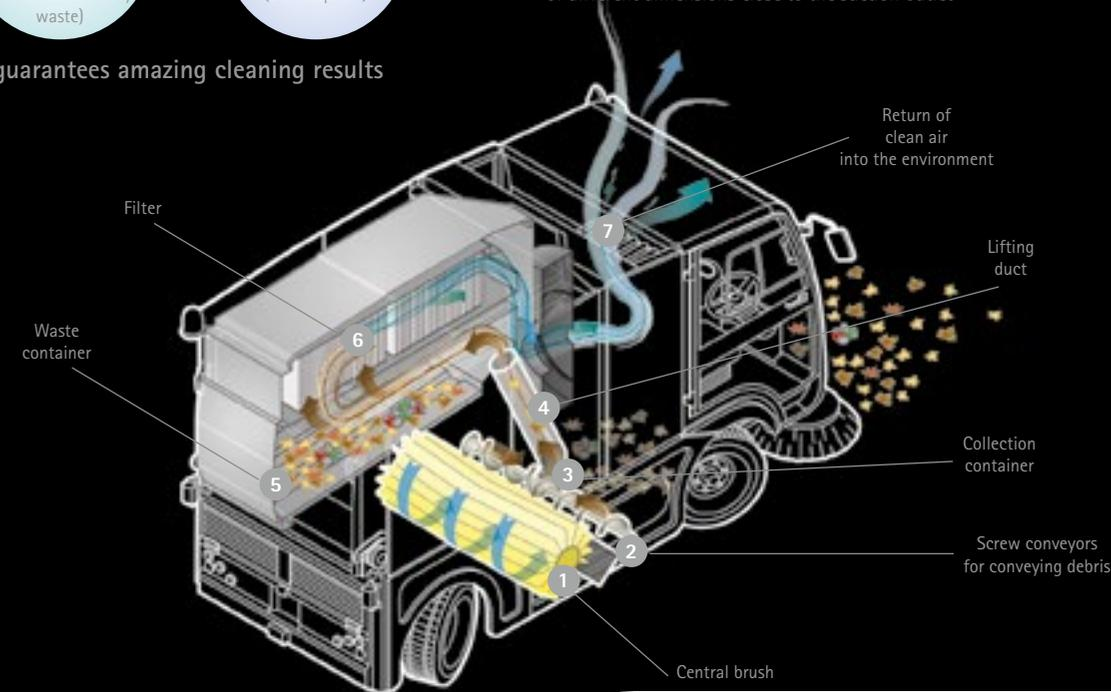
FIMAP<sup>4</sup> Twin Action changes the whole concept of cleaning: the cleaning action is concentrated only on the central brush
