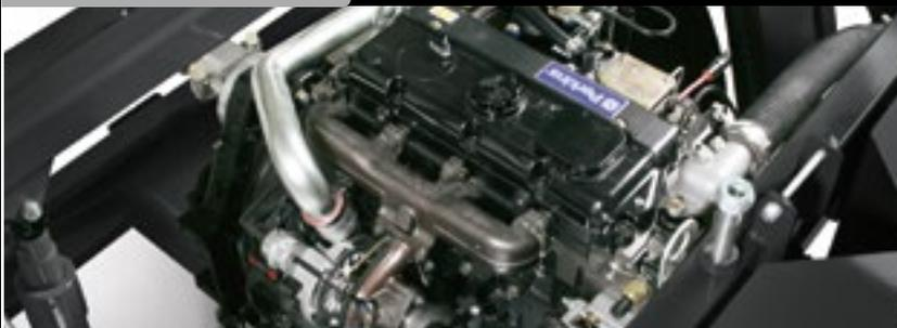
The engine, manufactured by PERKINS, delivers 100HP (75 KW) at only 2200 rpm with maximum torque of 1400 and 4400 cc displacement.
