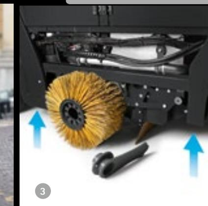
Fimap has produced a special device to control the vehicle height from the ground which, acting separately on the four wheels, maintains constant the height from the ground, optimizing work and stability. This device can also maintain the height of the vehicle unchanged even when the load varies. The operator can position the machine on three different pre-established levels in order to meet various needs.
