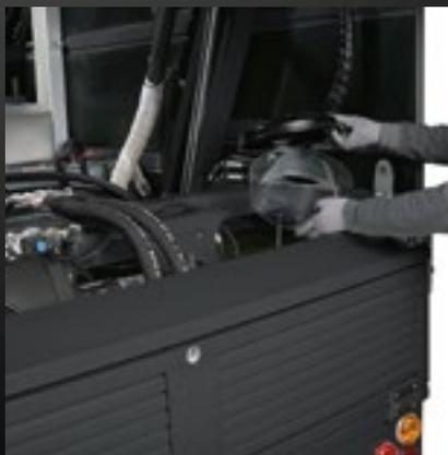
The engine air filter and the hydraulic oil radiator are located in the rear of the machine and can be accessed by means of a door which can be opened even with the hopper lowered. This position has been chosen to keep these parts exposed to a flow of clean air in order to avoid clogging and overheating and to reduce the possibility of damage.
