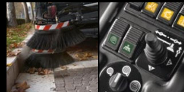
The side brushes can be equipped with special nozzles for spraying water (optional) which are effective for controlling dust during sweeping
